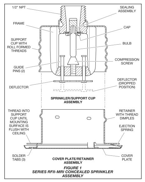
below. Down drafts through the Sprinkler/Support Cup Assembly can delay sprinkler operation in a fire situation.
