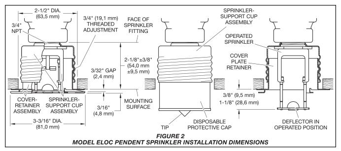
Step 2. Remove the Protective Cap.
