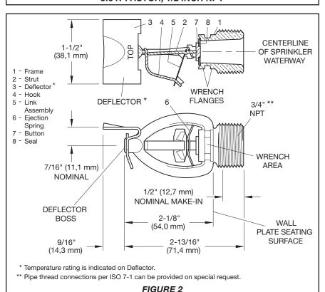
SERIES TY-FRL (TY4322) EXTENDED COVERAGE HORIZONTAL SIDEWALL SPRINKLERS 8.0 K-FACTOR, 3/4 INCH NPT
