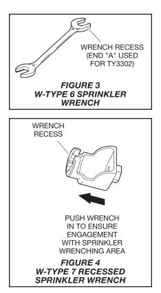
Care must be exercised to avoid damage to the sprinklers before, during, and after installation. Sprinklers damaged by dropping, striking, wrench twist/slippage, or the like, must be replaced. Also, replace any sprinkler that has a cracked bulb or that has lost liquid from its bulb. (Ref. Installation Section).
