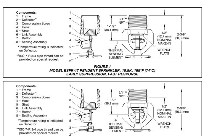
FIGURE 2 MODEL ESFR-17 PENDENT SPRINKLER, 16.8K, 212°F (100°C) EARLY SUPPRESSION, FAST RESPONSE
