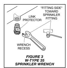
Step 2. Wrench-tighten the Model ESFR-17 Sprinkler using only the W-Type 35 Sprinkler Wrench as shown in Figure 3, and by fully engaging (seating) the wrench on the sprinkler wrench flats as shown in Figures 1 and 2.
