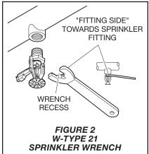
**Step 3.** Apply a W-Type 21 Sprinkler Wrench to the sprinkler by fully seating the wrench recess on the sprinkler wrench flats, see Figure 1.
