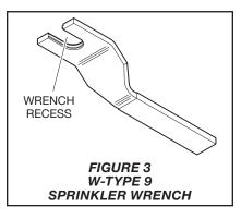
wrench twist/slippage, or the like, must be replaced. Also, replace any sprinkler that has a cracked bulb or that has lost liquid from its bulb, see Installation Section.
