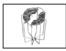
**Step 4.** Swivel the second clip to engage the open end onto the opposing bar and slide toward the base plates until fully seated against the base plates.
