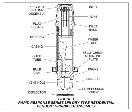
The system's water or air pressure is then able to unseat the Plug with Sealing Assembly. The Plug Spring turns the Plug with Sealing Assembly aside, allowing the sprinkler to activate and flow water.
